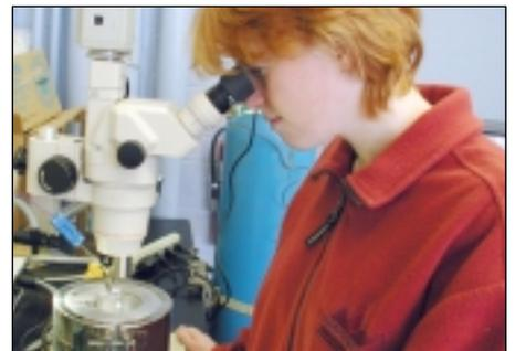
Marieke Rijkse, a visiting student from Delft University, observes the "sintering" process – a critical step in rotomolding, where polymer particles are heated and coalesce in a homogenous melt.
