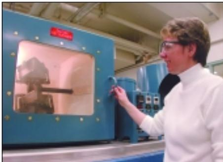
Lab Manager Elizabeth Takács demonstrates the rotomolding process. A weighed charge of plastic powder is placed in a mold, which is heated and rotated to distribute the powder evenly across the mold surfaces. As the powder melts, a homogeneous plastic layer forms on the surface of the mold. The mold is then cooled and the finished piece removed.
